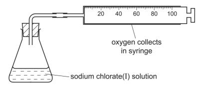
Sodium chlorate(I) is placed in the flask and 0.2 g of copper(II) oxide is added. This catalyses the decomposition of the sodium chlorate(I) and the volume of oxygen collected is measured every minute. The results are plotted to give a graph of the type shown below.
